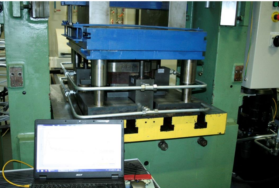
Tool for drawing with the blank-holder hydraulic control
